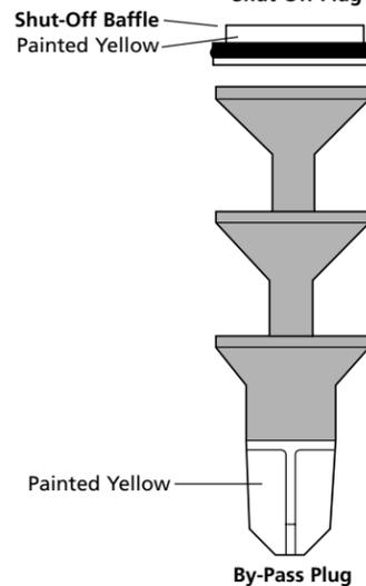
1. A Davis float shoe and float collar along with the Type 778 MC Stage Collar, are installed in the casing string and the casing is run to bottom. The yellow shut-off baffle is installed in the casing string at least (1) one joint above the Davis float collar. If API threads are run (8RD or Buttress) the baffle can be installed in the "J" section of a coupling. If premium threads are run, a separate baffle collar must be run.
