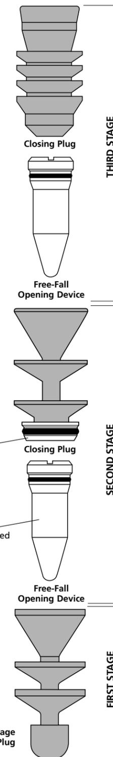
The Type 778 MC-3S stage collar is identified by its red markings and is always run as the lower of the two tools. Its free-fall opening device and closing plug are also identified by their red markings. The upper stage collar is always the Type 778 MC and the free-fall opening device and closing plug for it are standard.
