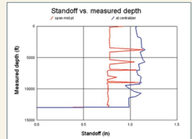
Davis will, on request, run a computer-analyzed program that will recommend centralizer placement and project casing stand-off. All that is required are some simple pipe and well data, including casing size, casing weight, casing seat, hole size, mud weight and, when deviation is present, full survey data, including kickoff point, rate of build and final deviation. Since centralization is most critical through the cemented interval, anticipated top of cement is also requested.
