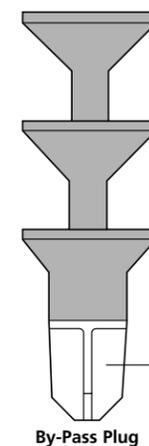
In this application, the by-pass plug follows first-stage cement and it is advisable to run a minimum of two joints between the float shoe and float collar.
